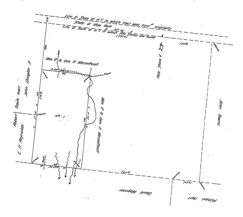
Draft of a tract of land situated in Scott Township in Wayne County, containing 81° 22°, and allowance of six per cent for roads &c. Surveyed for Horatio Benjamin on the 18<sup>th</sup> day of June A.D. 1873; being a part of a larger tract of 435° 56° and allowance; originally surveyed on a Warrant to John Craig, dated the 1<sup>st</sup> day of July 1784.
